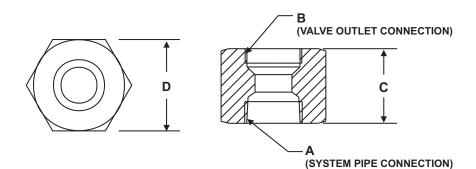
**Note:** For direct connection of cylinder valve to distribution piping.
