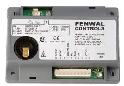
The 35-40 series of direct spark gas ignition controls operates on either 12 or 24 VDC. Over the past few years, we have received increased request from OEMs to provide DC controls with all the features typically found in our AC powered controls. As appliances become more advanced and they increase the amount of electronics within, they have increased components and boards that operate on
