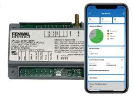
What does ConnectedControls do for me? Integrates into your appliance collecting data from the gas ignition control and other sensors to monitor performance. Standard data is stored and trended to monitor performance goals such as flame strength quality, while critical data is transmitted to end-users and service personnel to alert them of conditions like ignition lockout so immediate action can be taken for resolution.
