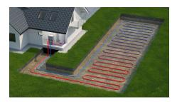
Geothermal Heat Pumps extract the ground's consistent heat, which remains relatively constant below 10 feet deep. Geothermal heat pumps transfer the heat from the ground into buildings for heating and reverse the process in the summer. Geothermal heat pumps are considered one of the most energy-efficient, environmentally clean, and cost-effective systems for heating and cooling buildings.
